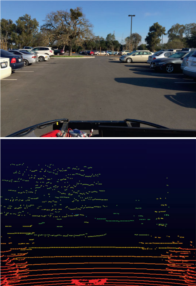
Fig. 5.3 Above: a driving scene with parked cars. Below: the view from a laser scanner
