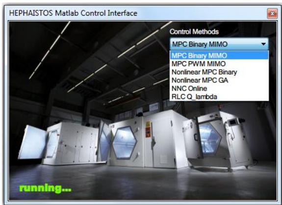
Figure 2.16. Remote control interface of HEPHAISTOS.
