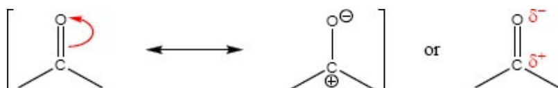
Scheme 1.1.1: Carbonyl group resonance structures and equivalent notation, explicitly showing the bond polarity with partial charges.
