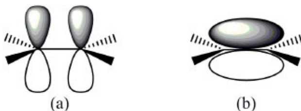
Figure 1.1.1: A simplified representation of the spatial distribution of two adjacent p orbitals (a) and their combination into a \pi bond (b) between two sp^2 carbon atoms. The \pi -bonds in a triple bond would be along orthogonal planes to each other.
