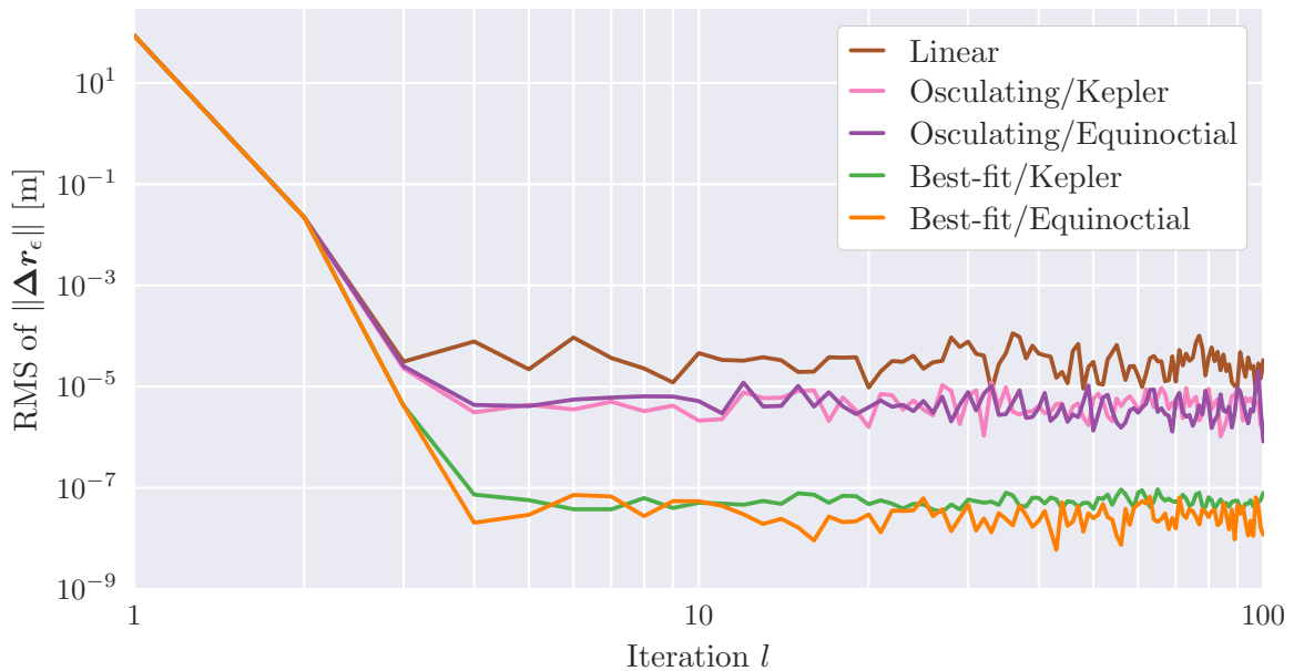
Figure 7.4: Simulated data. RMS of 3D coordinate difference \|\Delta\mathbf{r}_\epsilon\| for a complete arc after each iteration l .
