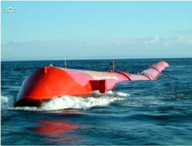
Figure 8.18 WEC concept and demonstration unit (Source: Pelamis Wave Power Ltd.).
